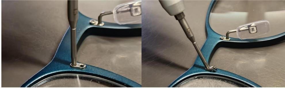
If the nose pad arm is broken at the base, it can be difficult to remove. Try to pry it off with the T5 screw bit. If the base comes loose, the frame can be repaired. However, if the base breaks without the part coming loose, the frame cannot be repaired.
