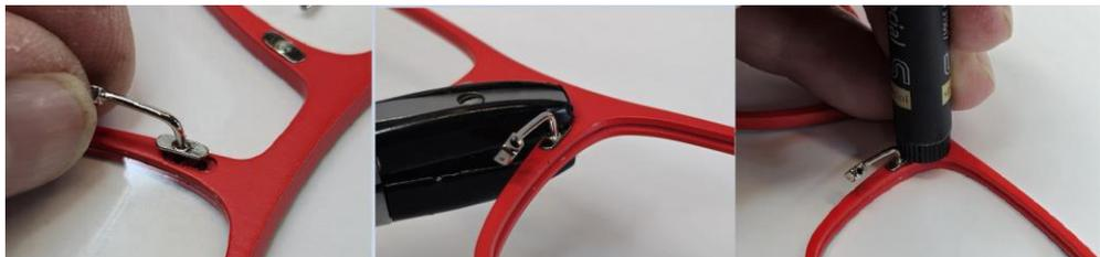
The thread locker will achieve full bond strength in approximately 30 minutes. The curing process will be complete in 24 hours.
