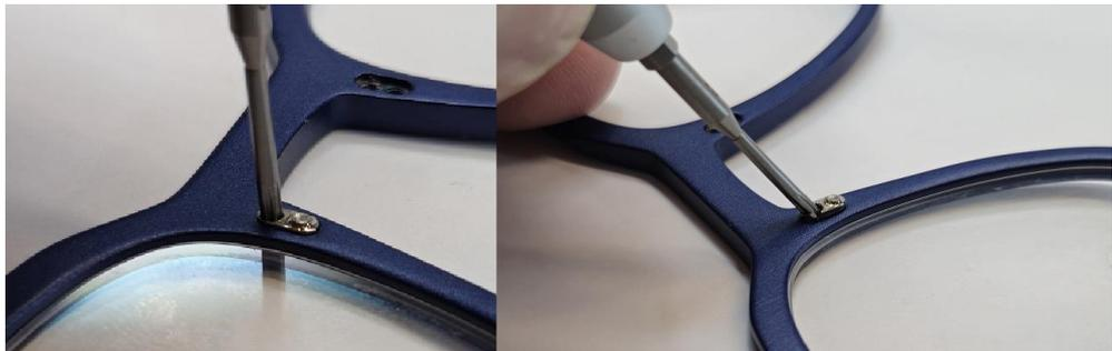
Remount the Nose pad arm with T3 screw:
