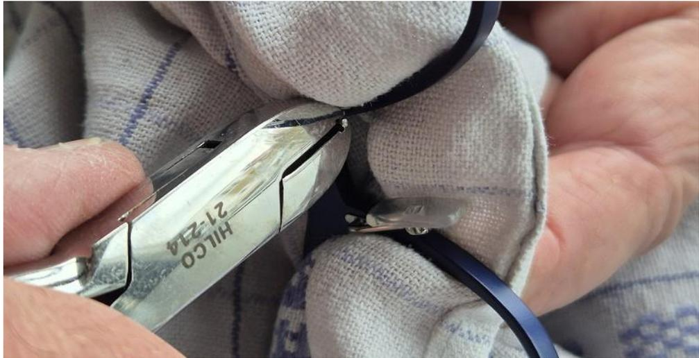
If it is a cold solder and the nose pad arm is missing, keep a firm grip and apply pressure while unscrewing the T3 screw. Use the T5 screw bit, place the tip of the T5 bit in the screw hole, and pry off the nose pad arm base plate.
