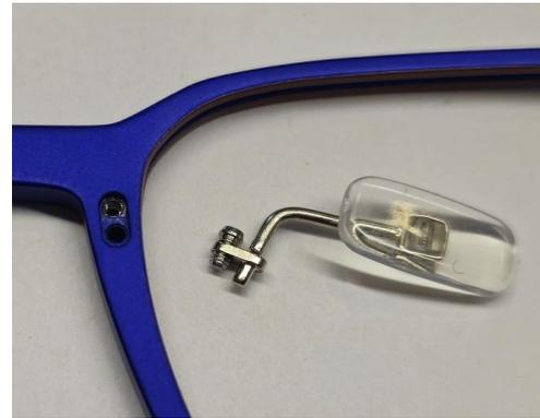
Defect nosepad screws (PP39)
