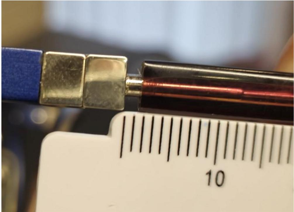
Heat and straighten the ear bend. Wriggle off the temple sleeve from the temple core.
