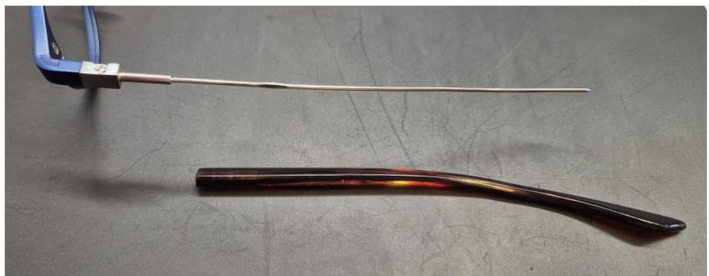
Add 2mm to the measure of the shrinkage and cut off the end of the temple core.
