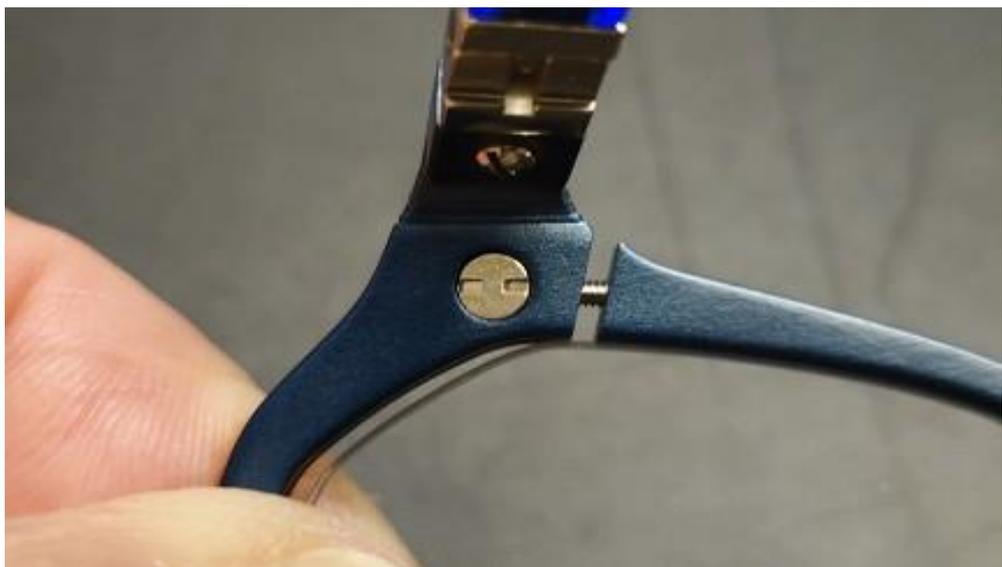
Mount the lens and tighten the rimlock screw.
