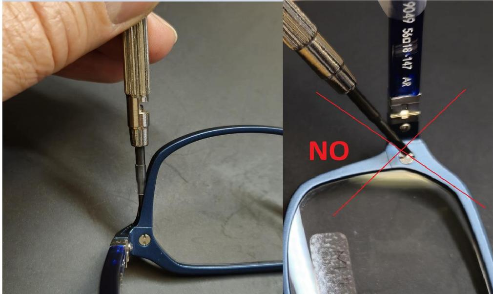
Do not unscrew the rimlock screw completely. Only so it is enough to unmount and remount the lenses.
