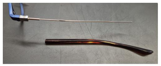
Add 2mm to the measure of the shrinkage and cut off the end of the temple core.
