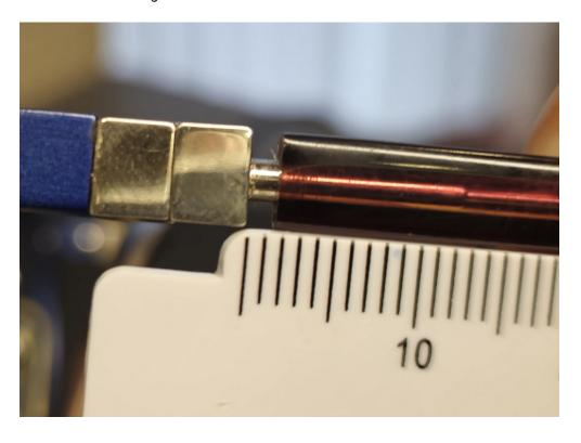
Heat and straighten the ear bend. Wriggle off the temple sleeve from the temple core.
